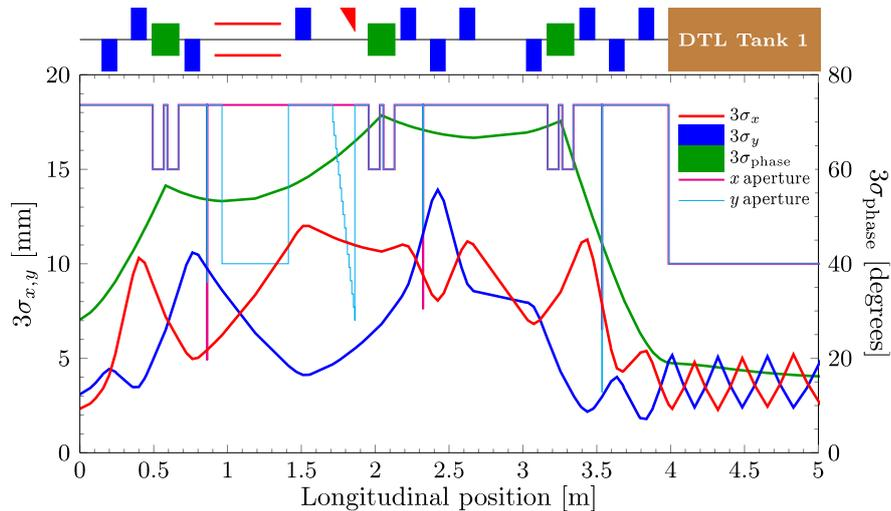
Figure 1: Schematic layout (top) and beam envelopes with apertures (bottom) for MEBT.
