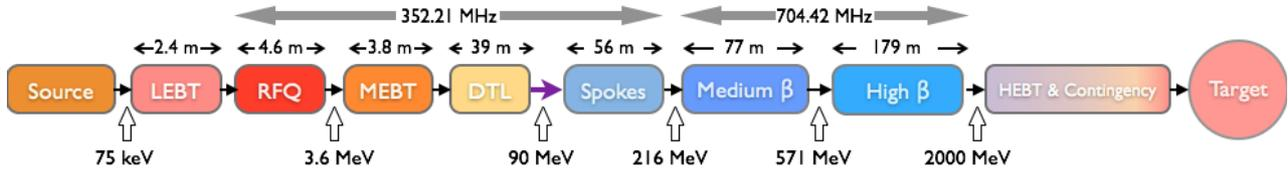
Figure 1: The overall layout of the different sections of the ESS linac. The front end including the spoke cavities run at 352.2 MHz, while the elliptical cavities run at twice that frequency. The beam energy at each intersection is given below the intersections.
