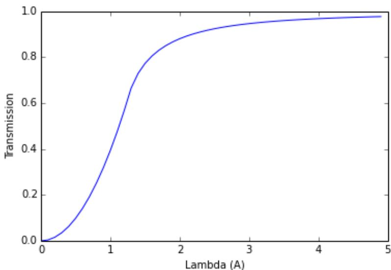
Figure 7: Transmission curve of an example bender for 150 m instruments to transmit 2Å neutrons.
