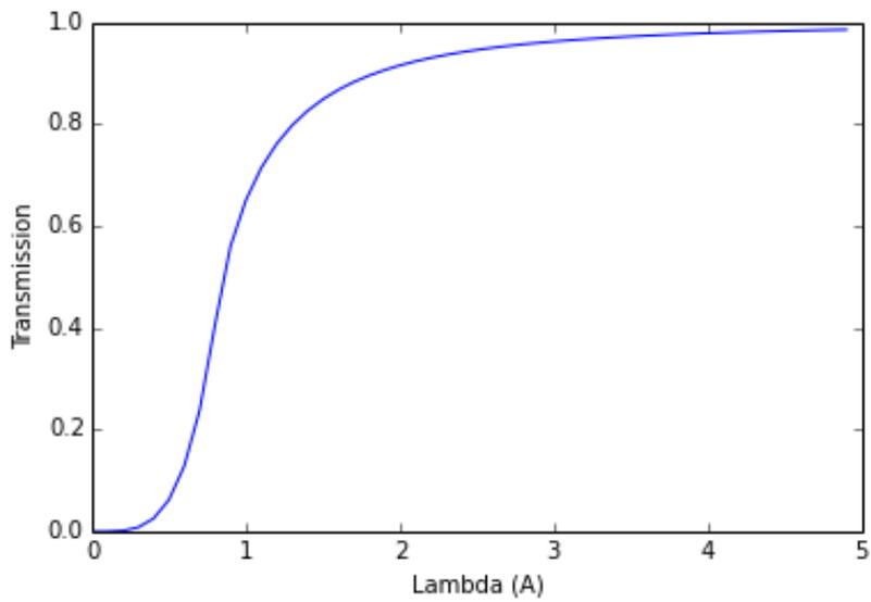
Figure 4: Transmission of a generic, curved 150 metre guide system as described in the text compared to a straight one, neglecting reflectivity losses.
