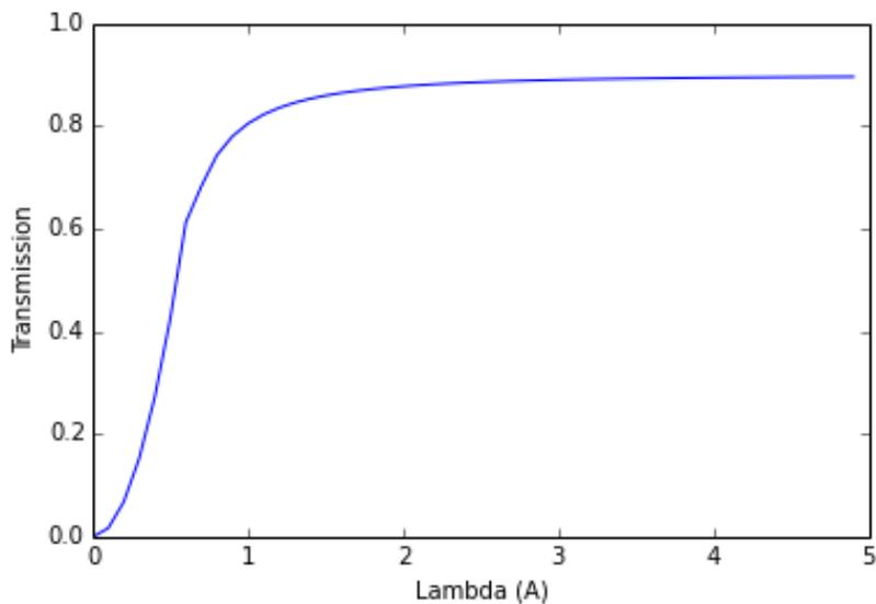
Figure 8: Transmission curve of an example bender for 60 m instruments to transmit 1Å neutrons.
