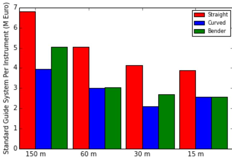
Figure 10: Cost of each instrument using the standard ESS guide concept, to isolate the cost delta for the different curving options (therefore omitting the baseline suite).
