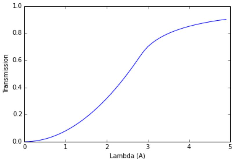
Figure 9: Transmission curve of an example bender for 60 m instruments to transmit 4 Å neutrons.
