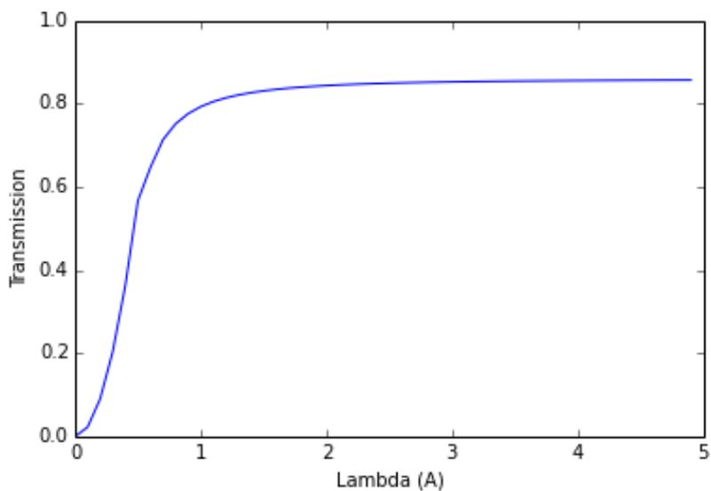
Figure 6: Transmission curve of an example bender for 150 m instruments to transmit 1 Å neutrons.
