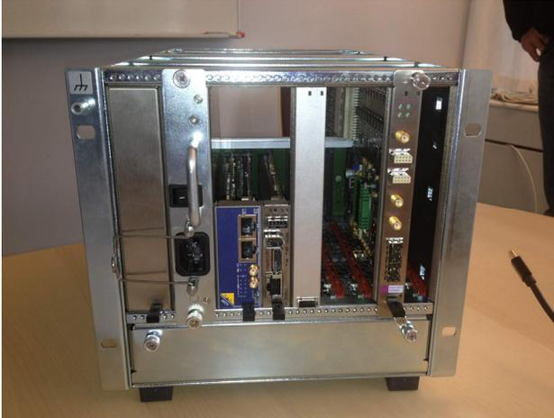
Figure 3: Picture of the prototype MTCA.4 system.
