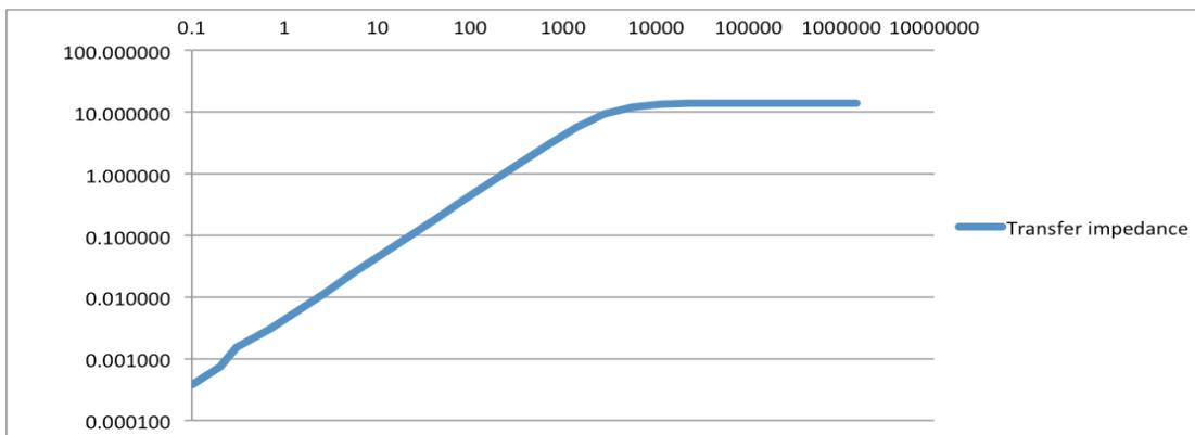
Figure 3: frequency response of the BPM transfer impedance. The horizontal axis is the frequency in MHz and the vertical one is the transfer impedance in Ohm. The working frequency (352 MHz in this case) is lower than the cut-off, resulting in an overall capacitive behaviour.
