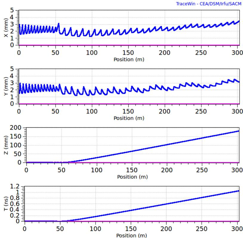
Figure 4: calculated bunch sizes in the superconducting linac along the x, y and z axis with no powered cavity after the spokes. Calculations by: R. Miyamoto (ESS, Beam Dynamics group)
