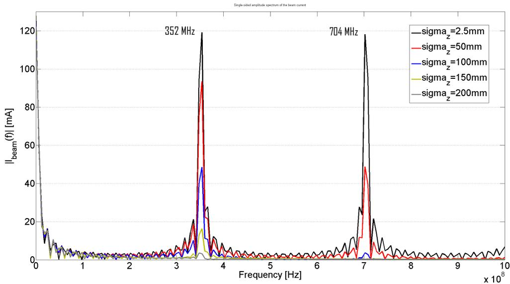
Figure 5: amplitude reduction of the beam current harmonics as a result of de-bunching.
