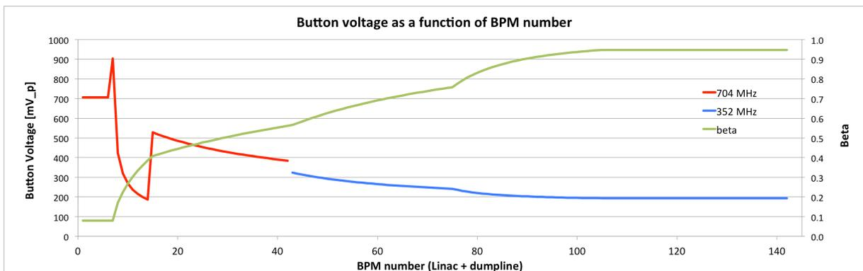
Figure 2: button voltage with button diameters of 24 mm and 40 mm for the beam pipe apertures of 60 mm and 100 mm respectively.
