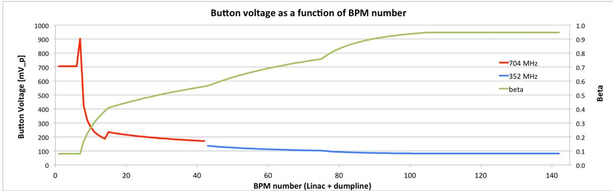
Figure 1: calculated button voltage as a function of BPM number. The dumpline section is added to the end of the linac. The exponential-like decays are due to the increase of the beam velocity and the sharp changes are mainly due to the variations in the beam pipe and button diameters. The processed frequency is 704 MHz in the spokes and the upstream sections and 352 MHz in all the other sections.
