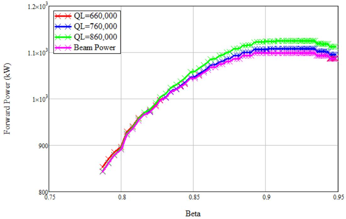
Figure 5. Required peak forward power as a function of loaded  $Q$  ( $Q_L$ ).
