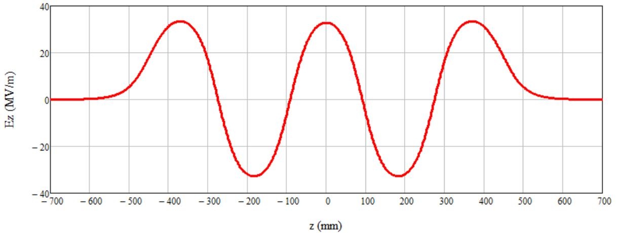
Figure 2. Five cell high beta field profile with  $\beta_g=0.86$ , a peak surface field of 40 MV/meter, and a stored energy of 128 J.
