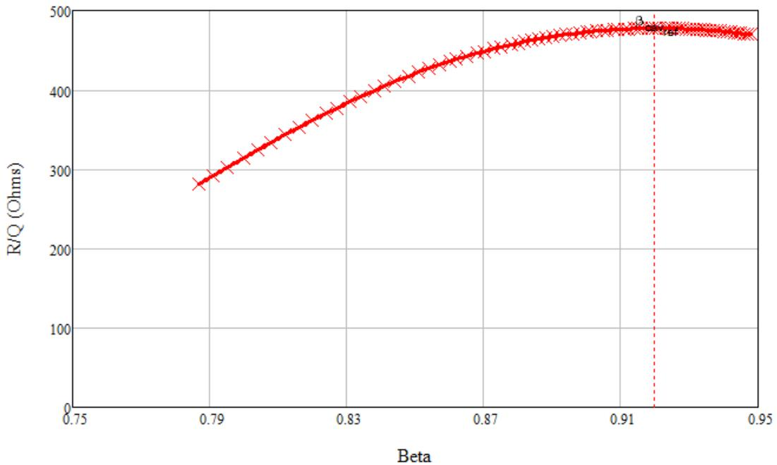
Figure 3. R/Q plot for the 5 cell High Beta Cavities. The maximum acceleration R/Q of 478 Ohms occurs at a  $\beta$  of 0.92 for cavity 53 (first cavity in the fourteenth cryomodule)
