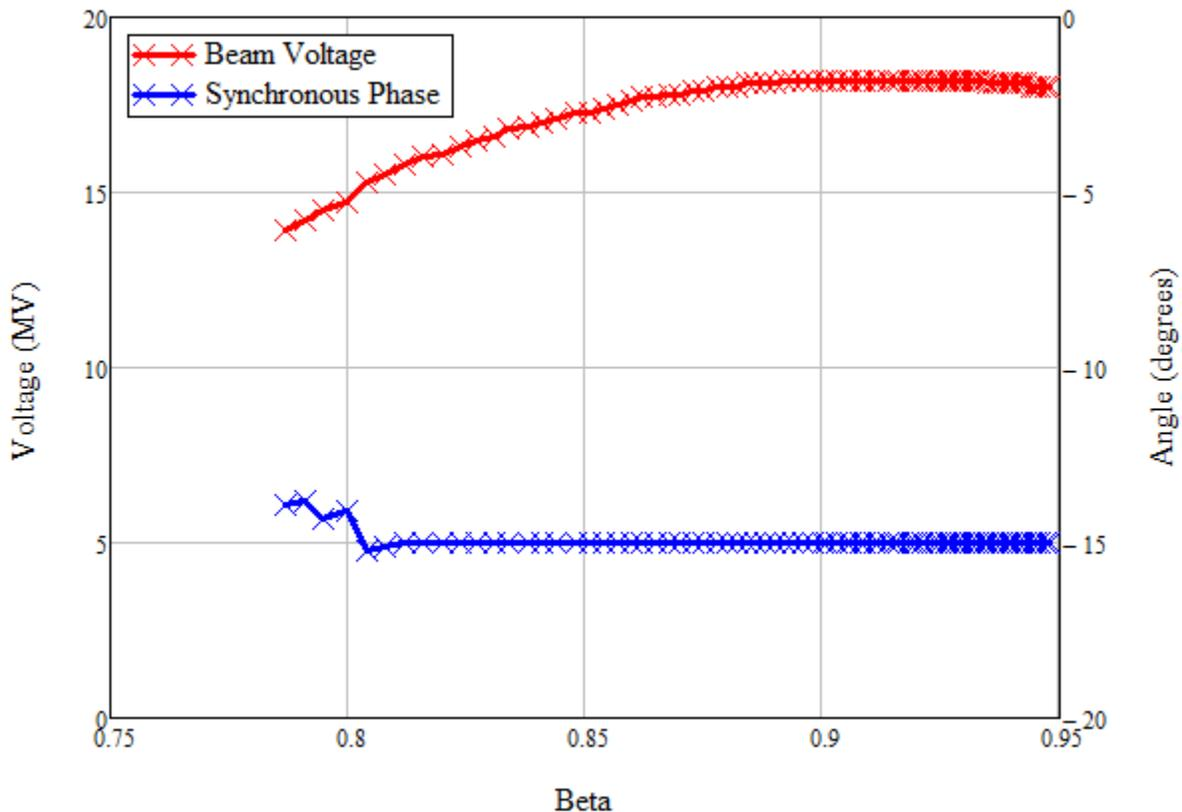
Figure 1. Beam Voltage and Synchronous Phase for the High Beta Section of the ESS OPTIMUS Lattice.
