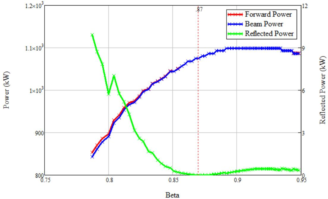
Figure 4. Forward and reflected power for the High Beta cavities with a  $Q_L$  of  $657 \times 10^3$ . The  $Q_L$  was chosen for the operating point of  $\beta=0.87$  and a beam current of 62.5 mA.
