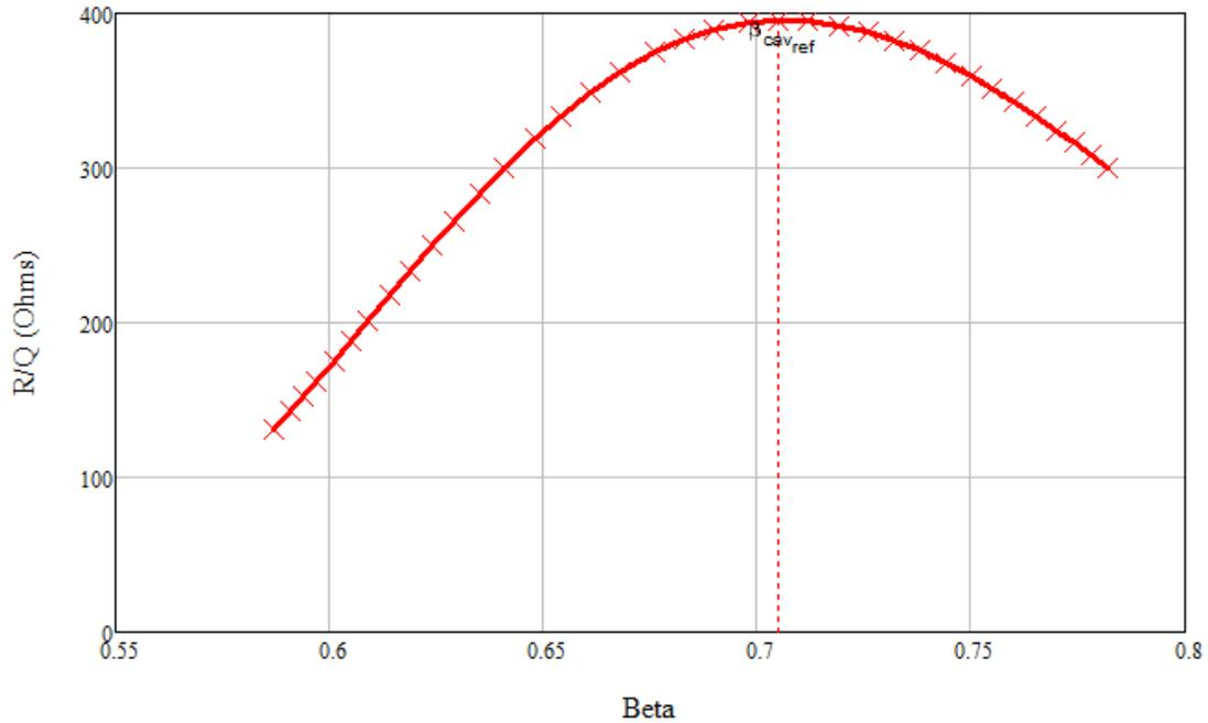
Figure 3. R/Q plot for the 6 cell Medium Beta Cavities. The maximum acceleration R/Q of 395 Ohms occurs at a  $\beta$  of 0.705 for cavity 22(second cavity in the fifth cryomodule)
