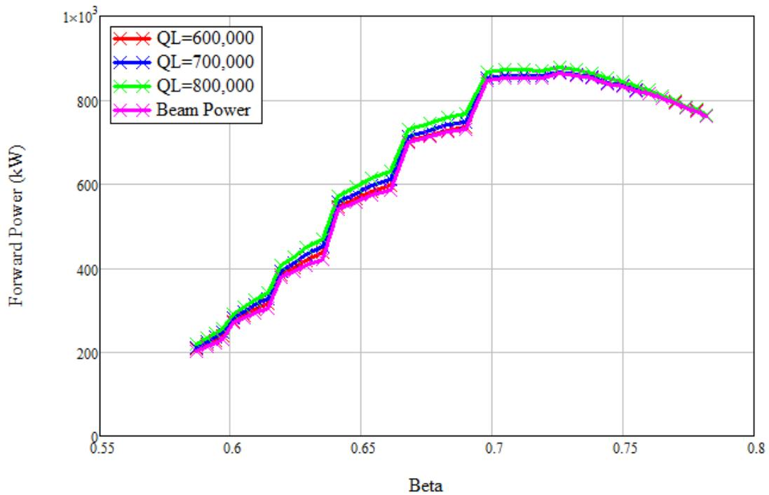
Figure 5. Required peak forward power as a function of loaded  $Q$  ( $Q_L$ ). At  $\beta=0.705$ , a  $Q_L$  of 700,000 requires 0.7% more power and  $Q_L$  of 800,000 requires 2% more power than the power required with  $Q_L$  of 600,000.
