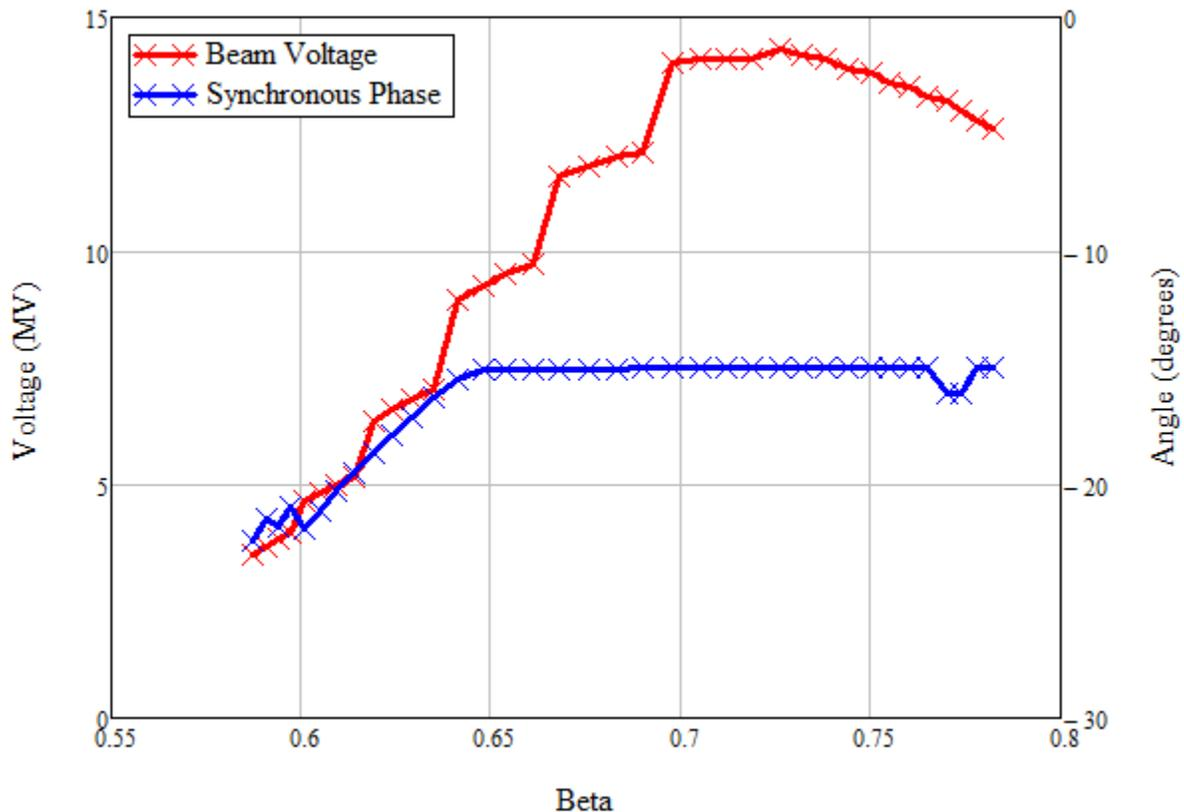
Figure 1. Beam Voltage and Synchronous Phase for the Medium Beta Section of the ESS OPTIMUS Lattice.
