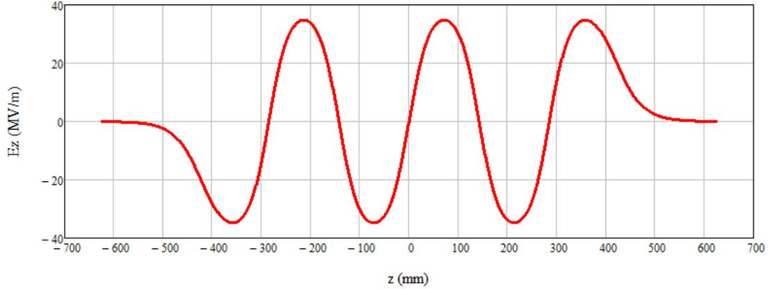
Figure 2. Six cell medium beta field profile with  $\beta_g=0.67$ , a peak surface field of 44 MV/meter, and a stored energy of 144 J.
