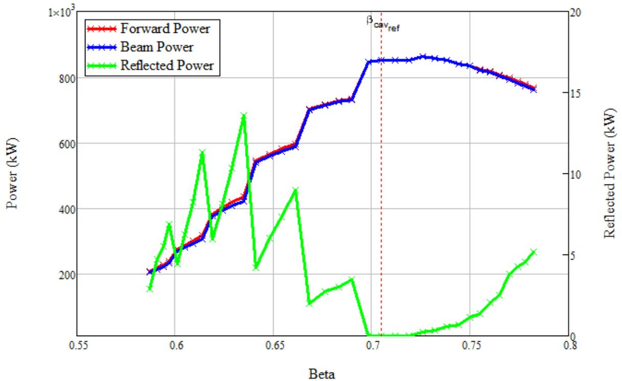
Figure 4. Forward and reflected power for the Medium Beta cavities with a  $Q_L$  of  $590 \times 10^3$ . The  $Q_L$  was chosen for the operating point of  $\beta=0.705$  and a beam current of 62.5 mA.
