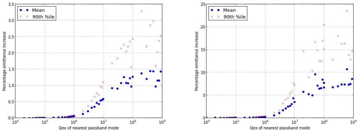
Figure 4:  $Q_{ex}$  scan for a 5-cell (left) and 6-cell (right) lattice with 0.5%/0.5° injection errors. Blue points indicate the average emittance for the simulated linacs, while the red crosses show the 90th percentile.
