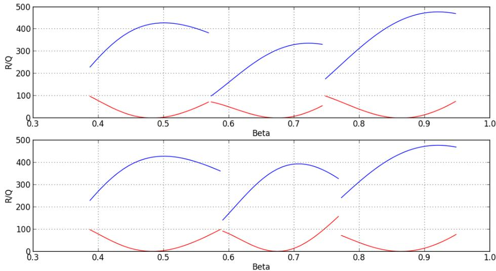
Figure 5: R/Q of the accelerating mode (blue) and passband mode (red) for the 5-cell linac (top) and 6-cell linacs (bottom) simulated in this note.
