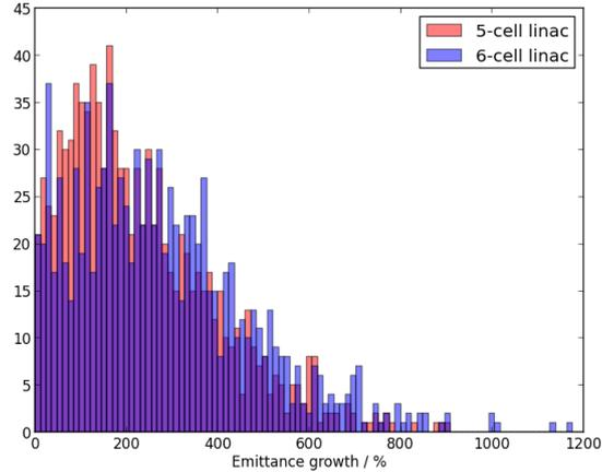
Figure 3: Distribution of simulated emittances for the two linacs.
