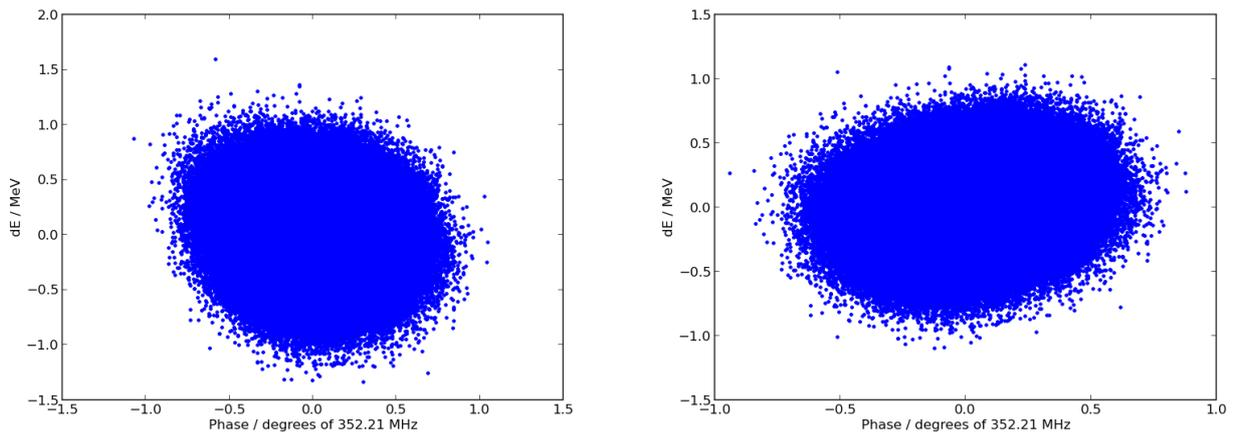
Figure 2: Bunch distribution in longitudinal phase space at the end of the 5-cell (left) & 6-cell (right) linacs for a beam with 0.5%/0.5° DTL-RF errors, but no passband modes or RF errors in the remainder of the linac.
