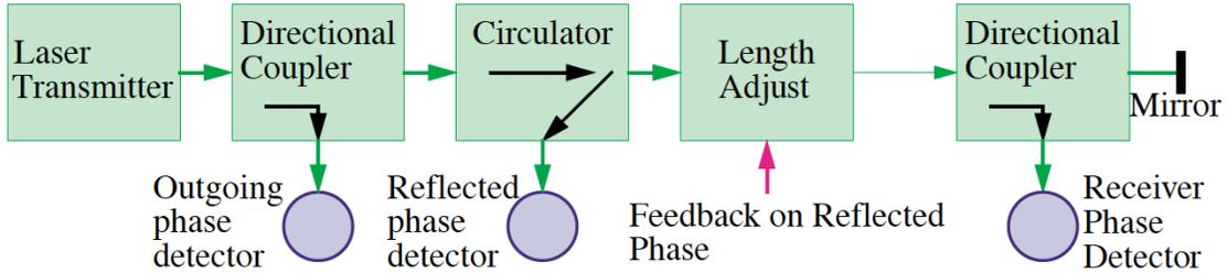
Figure 7: Typical phase drift compensation scheme for optical fiber[7]
