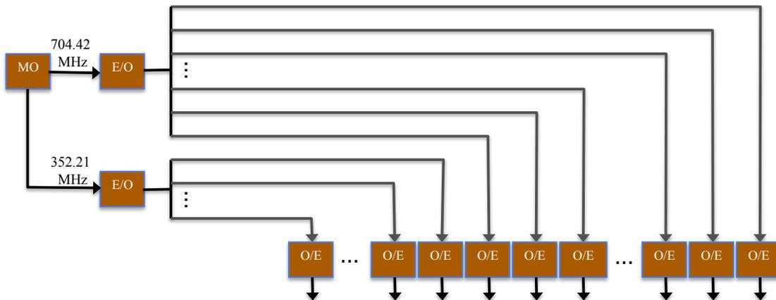
Figure 6: Schematic diagram for optical fiber based distribution
