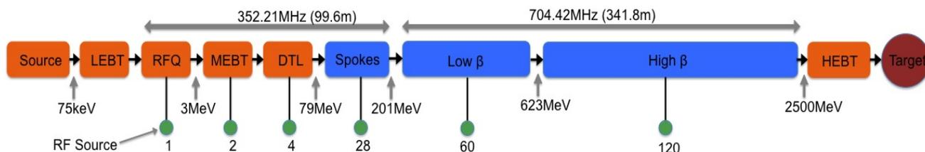
Figure 1: ESS Linac Layout and RF sources distribution
