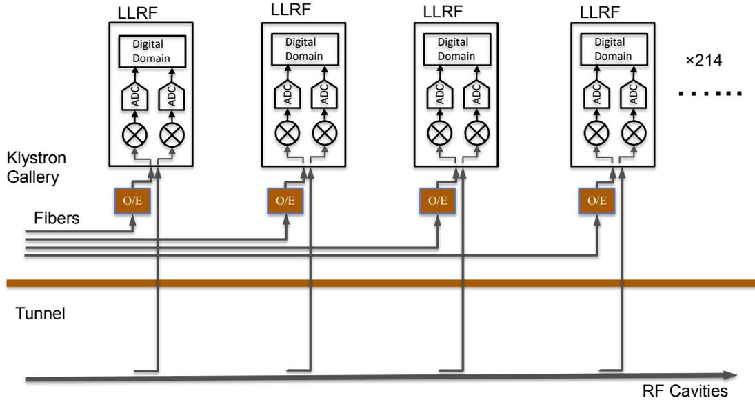
Figure 8: Local distribution in fiber based solution
