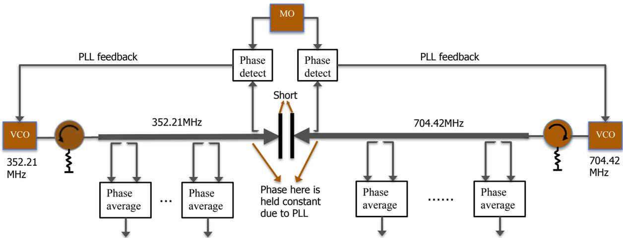
Figure 3: Phase drift control in main reference line by phase averaging
