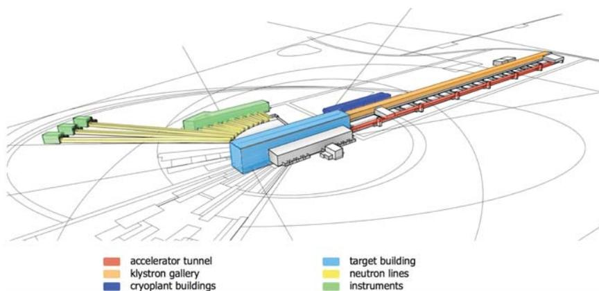
Figure 1: General layout of the ESS.
