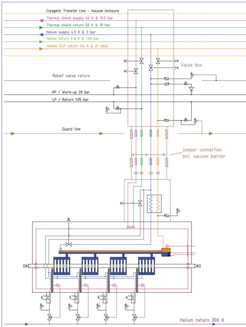
Figure 3: proposed schematic for the linac cryo distribution system.
