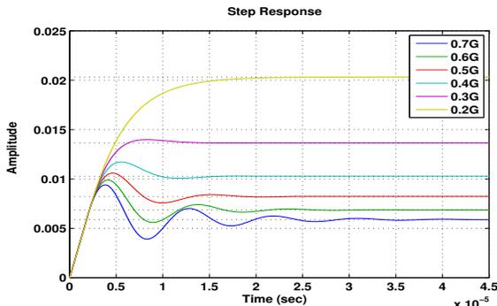
Figure 3: Closed loop noise suppression for superconducting cavity ( $G=241$ )
