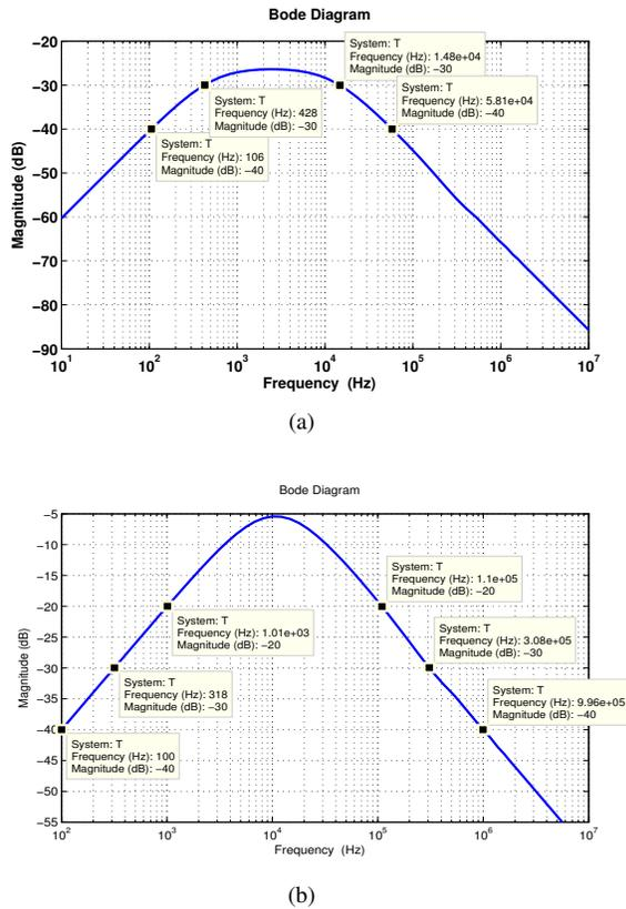
Figure 5: Noise suppression performance of PI feedback closed loop as a function of frequency for (a): superconducting cavity ( $K_p = 20, K_i = 2\pi \times 518$ ) and (b): normal conducting cavity ( $K_p = 1, K_i = 2\pi \times 10^4$ )
