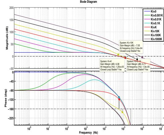
Figure 4: Phase margin reduced in open loop under different integral gains ( $2\mu\text{s}$  delay,  $K = 2\pi f_{hbw}$ )
