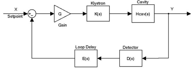
Figure 1: Block diagram of simplified feedback loop
