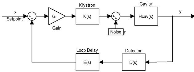
Figure 2: Block diagram of feedback loop with noise
