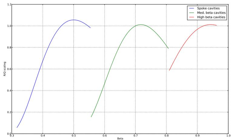
Figure 5: Scaling of the  $R/Q$  for each cavity in the linac.
