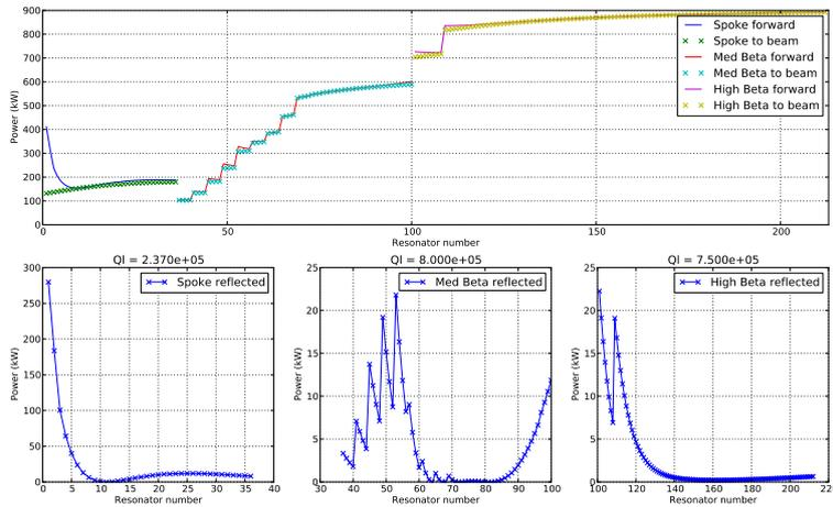
Figure 3: RF power for the unoptimised linac where the velocity dependence of the  $R/Q$  is included.
