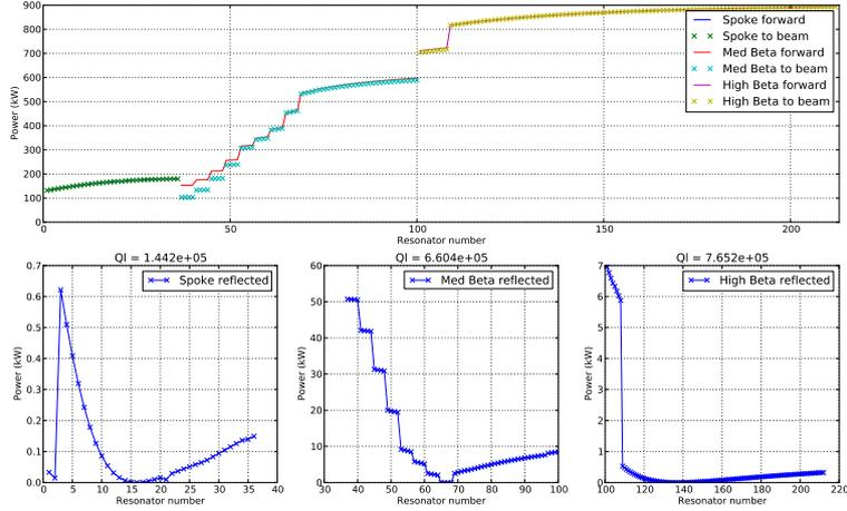
Figure 2: RF power for the optimised linac where the velocity dependence of the  $R/Q$  is ignored.
