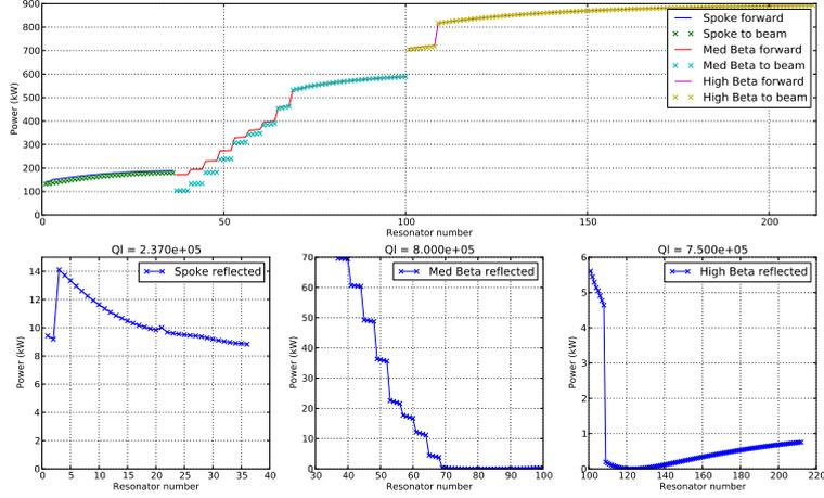
Figure 1: RF power for the unoptimised linac where the velocity dependence of the  $R/Q$  is ignored.
