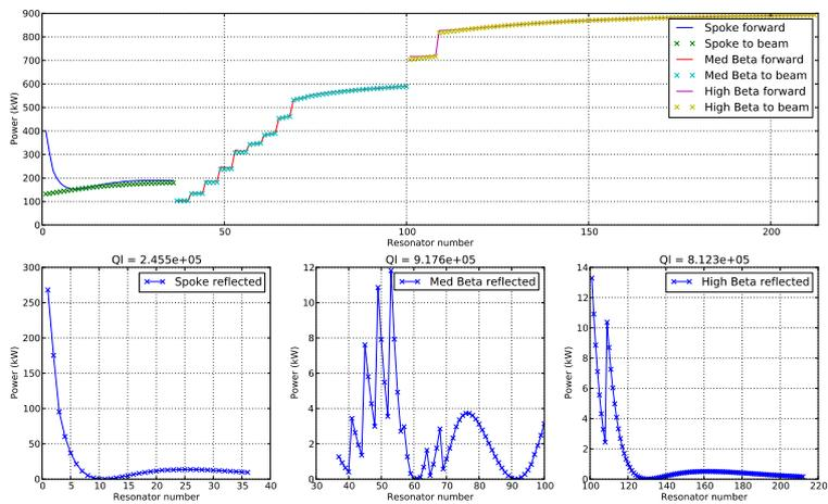
Figure 4: RF power for the optimised linac where the velocity dependance of the  $R/Q$  is included.
