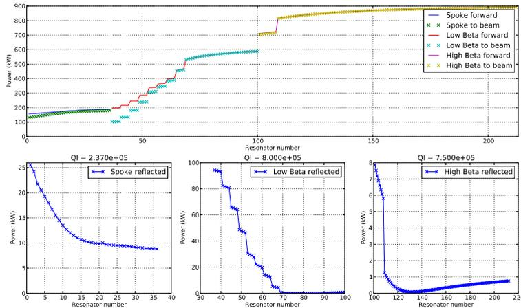
Figure 1: Forwarded and reflected power for the nominal coupler designs.
