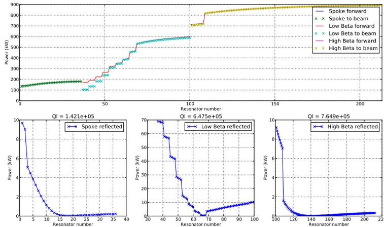
Figure 2: Forwarded and reflected power for optimised couplers.
