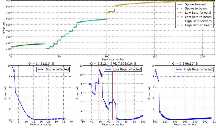
Figure 3: Forwarded and reflected power for the situation where three different coupler designs are used in the medium beta section.
