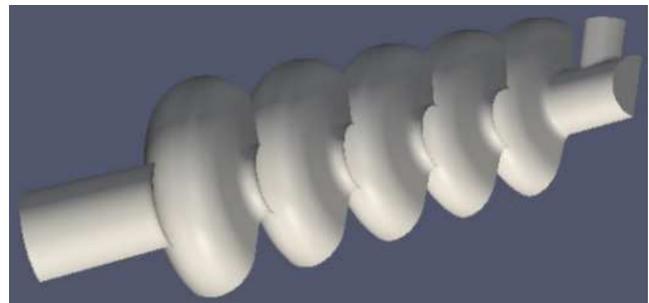
Figure 3: Elliptical cavity, with a high geometric  $\beta$  of 0.90.
