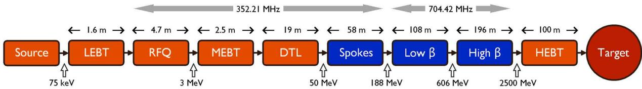
Figure 1: The “2011 hybrid” baseline layout of the ESS linac. Red sections – the RFQ, the DTL, and the Low-, Medium- and High- Energy Beam Transports, (LEBT, MEBT, and HEBT) – are normal conducting. Blue sections – spoke resonators, low- $\beta$ , and high- $\beta$  elliptical cavities – are superconducting.
