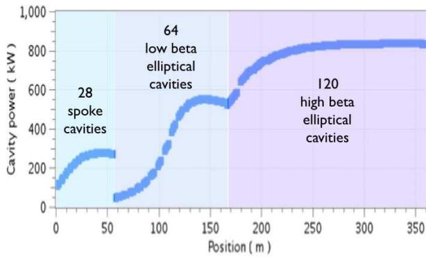
Figure 7: The power to beam of the superconducting part of the linac [26], as calculated from the lattice in [27].
