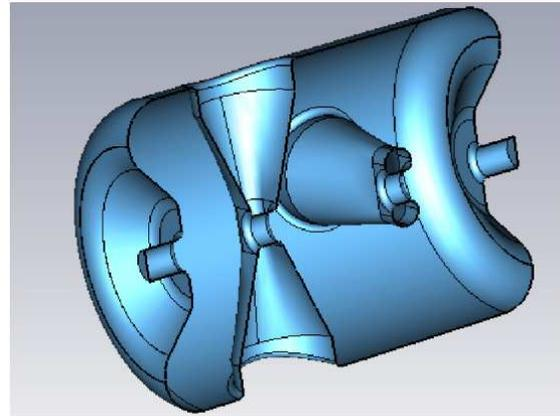
Figure 2: Double spoke resonator cavity, with an accelerating gradient of 8 MV/m and a geometric  $\beta$  of 0.57.
