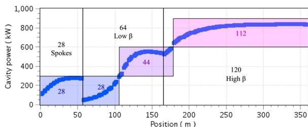
Figure 1: The supply of RF to each of the superconducting cavities in the Linac based on the hybrid layout presented in [3].
