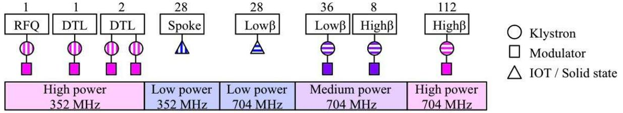
Figure 2: Layout of the RF power system for acceleration. Circles and squares represent klystrons respective modulators, while triangle represent IOT / Solid state amplifiers.
