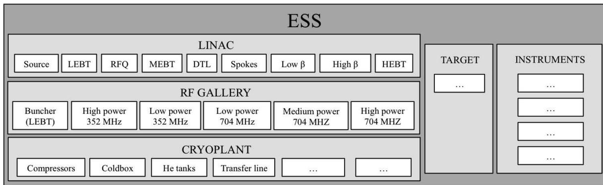
Figure 2: Schematic layout of the system structure.
