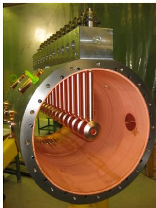
*Figure 2: Open DTL tank*
