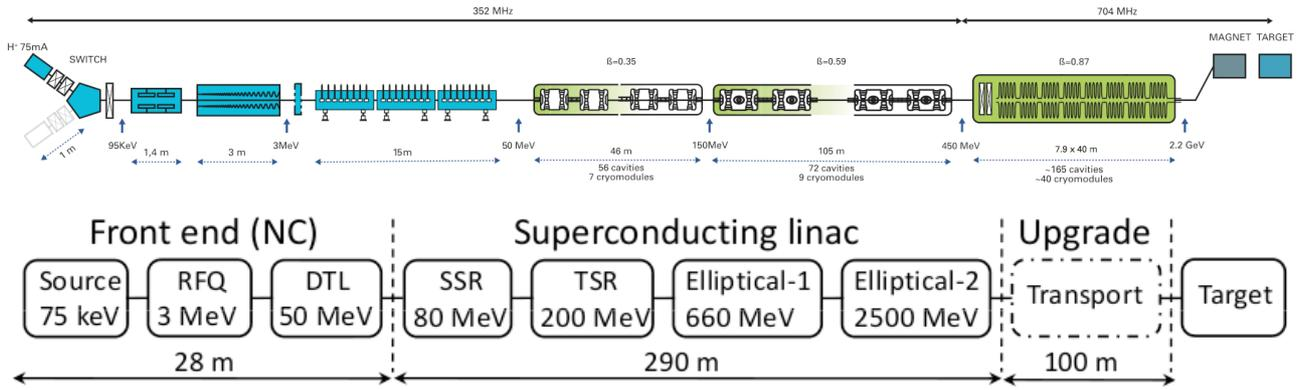
Figure 1: Block layout of the ESS linac. (TOP) The ESS-B layout, as it had evolved by the end of the *Initiative Workshop*, and as discussed at this conference [10]. (BOTTOM) A block diagram of the ESS-S layout, showing space in a “Transport” section that is reserved for a potential upgrade, in which additional cryomodules are installed to increase the beam power to 7.5 MW at a constant top energy of 2.5 GeV.
